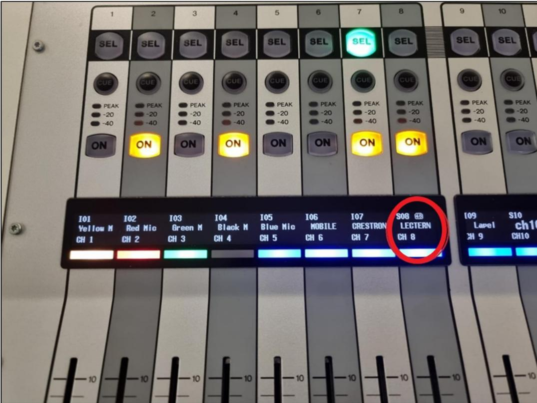
Laptop/Vivi volume is controlled by the slider labelled Crestron.
